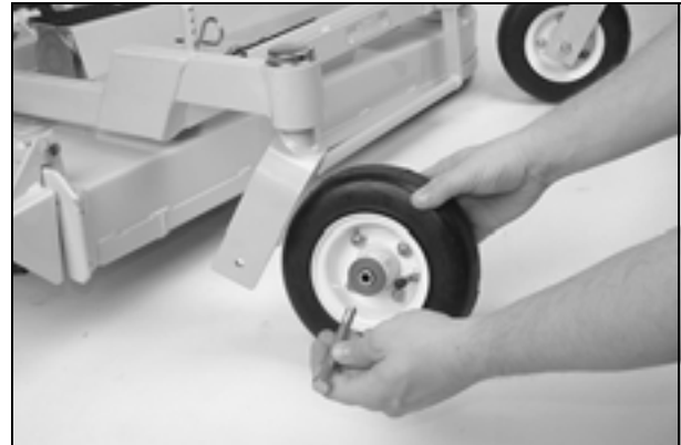
Deck Caster Wheel Installation
