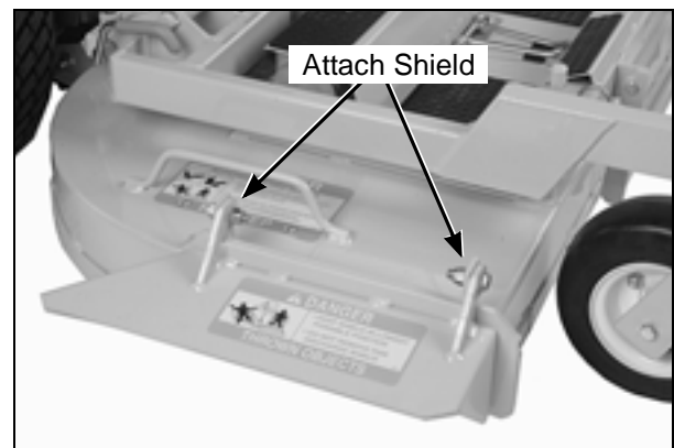
Deck Discharge Shield Installation
