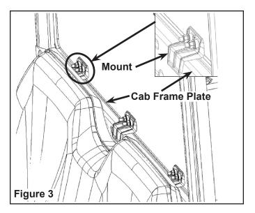
4. Clamp the mounts (PN 5439918) of rear panel on the cab frame plate. Figure 3.
