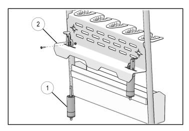
3. Insert tool rack ② into vehicle so that expansion anchors ① fully recede into vehicle receptacles as shown, then depress upper cams to lock in place. If installation is loose, remove tool rack from vehicle, tighten nuts at base of expansion anchors, and reinstall.
