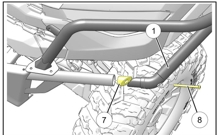
4. Fully insert threaded mount ⑦ and tapered fitting on LH upper bumper ① into existing bumper. Do not tighten screw at this time.
