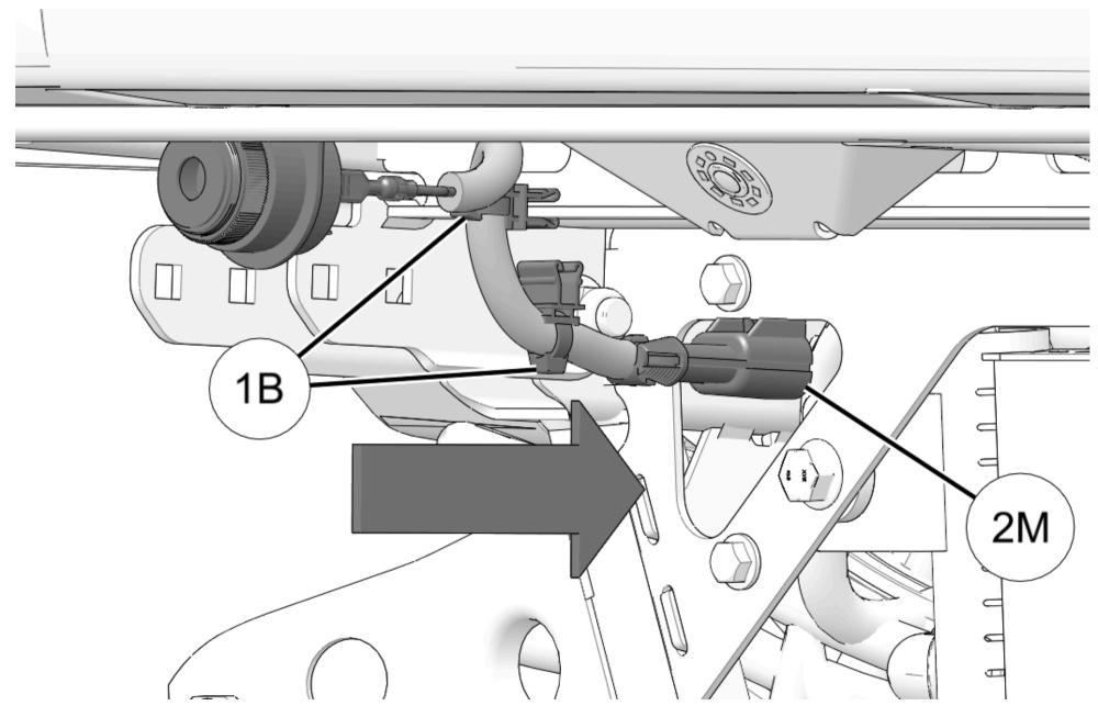
5. Locate reverse beeper connector (A) on main harness breakout. Remove connector from cap (B), then join to connector 2M to connector (A). Make sure adequate slack exists to permit full bed opening without harness tension.
