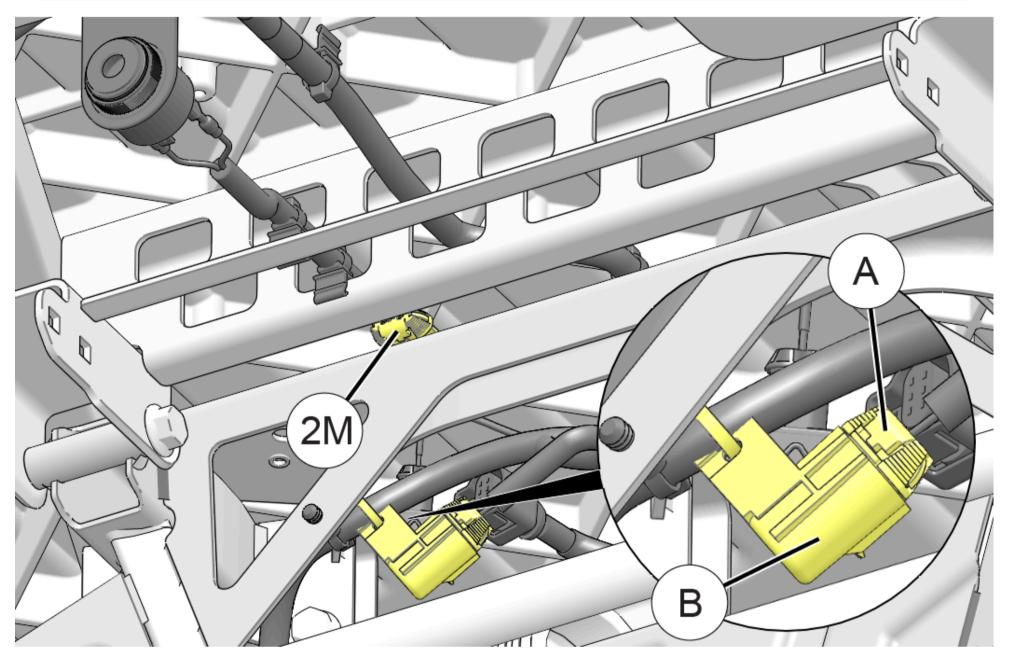
6. Slowly raise vehicle bed to ensure harness routing does not allow contact with hot components, sharp edges, or moving parts. If so, adjust routing and/or secure harnesses as required.
