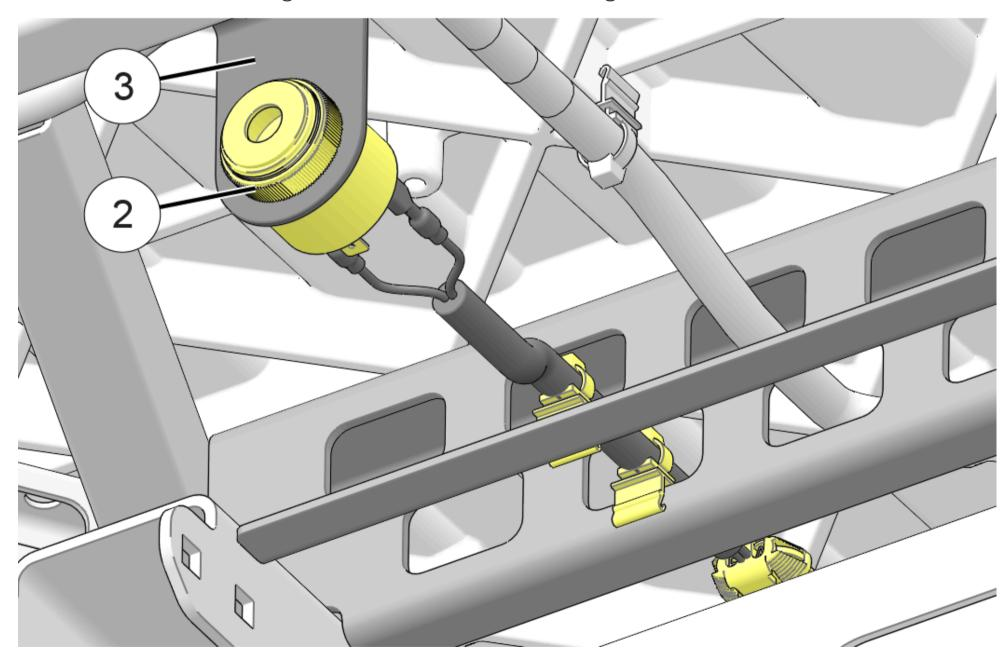
4. Route connector 2M rearward through openings in bed crossmember, then secure harness to crossmember using two edge clips 1B.
