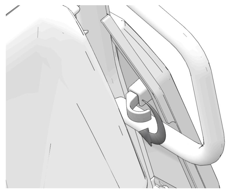
${\it 3. Install \, upper \, rocker \, panel \, with \, four \, retained \, push-pin \, rivets.}$
