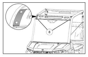
Torque lower windshield bracket mounting screws
