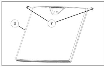
3. Put windshield assembly (3) in place on vehicle.
