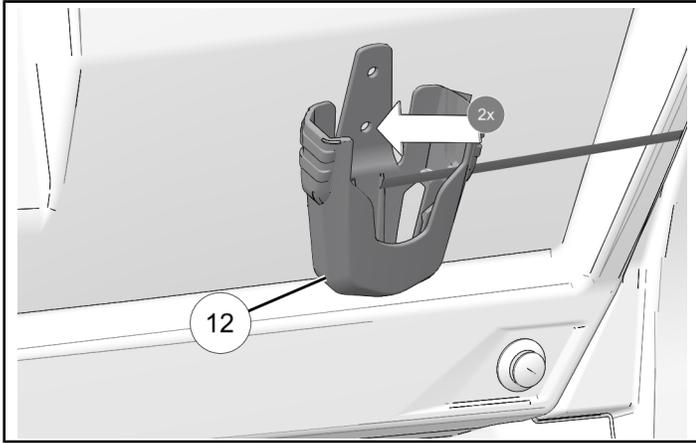
3. Install remote control mount ⑫ using two screws ⑭.
