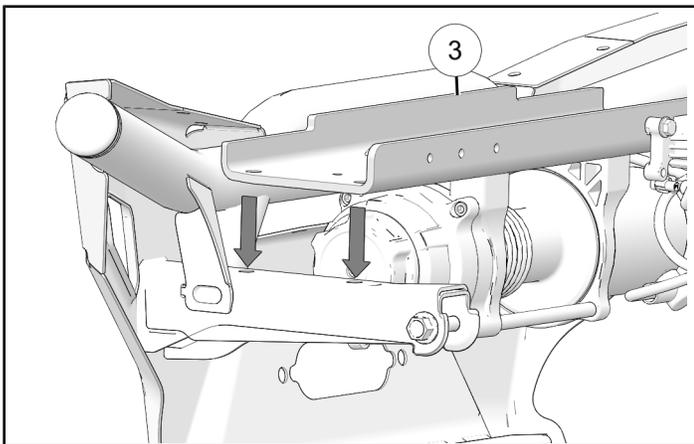
2. Install screws ⑨ into mounting plate ⑥. Make sure winch assembly ③ sits flush on bumper. Torque to specification.
