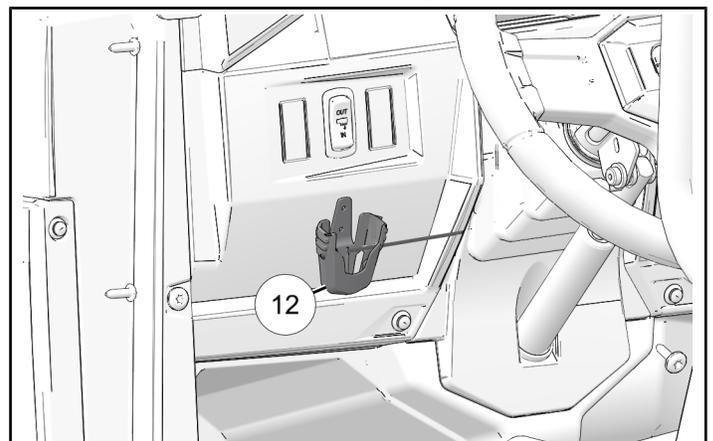
2. Locate and drill two holes. Use remote control mount ⑫ as a template to mark the holes.
