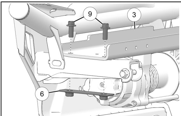
3. Install bumper on vehicle using kept screws and nuts (upper nut ⑧ not shown). Torque to specification.
