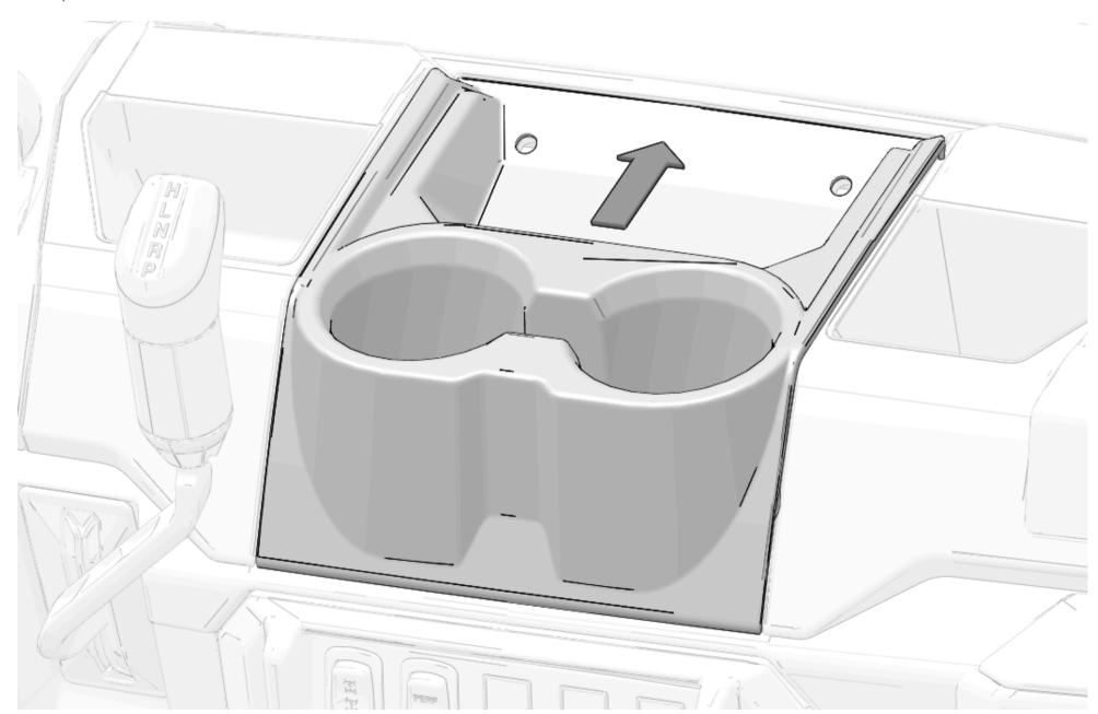
2. Install cup holder with two retained push-pin rivets.
