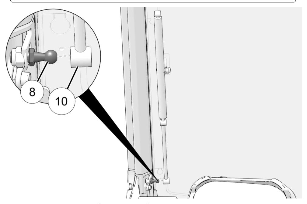
4. Open windshield and push upper shock cylinder 10 into upper ball fitting 8.
