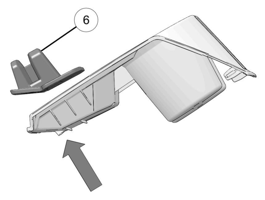
2. Use handle base (6) as a template to mark three holes on cup holder.
