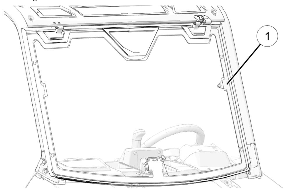
3. Move pin on left side windshield hinge into bushing on left side windshield mount 12.
