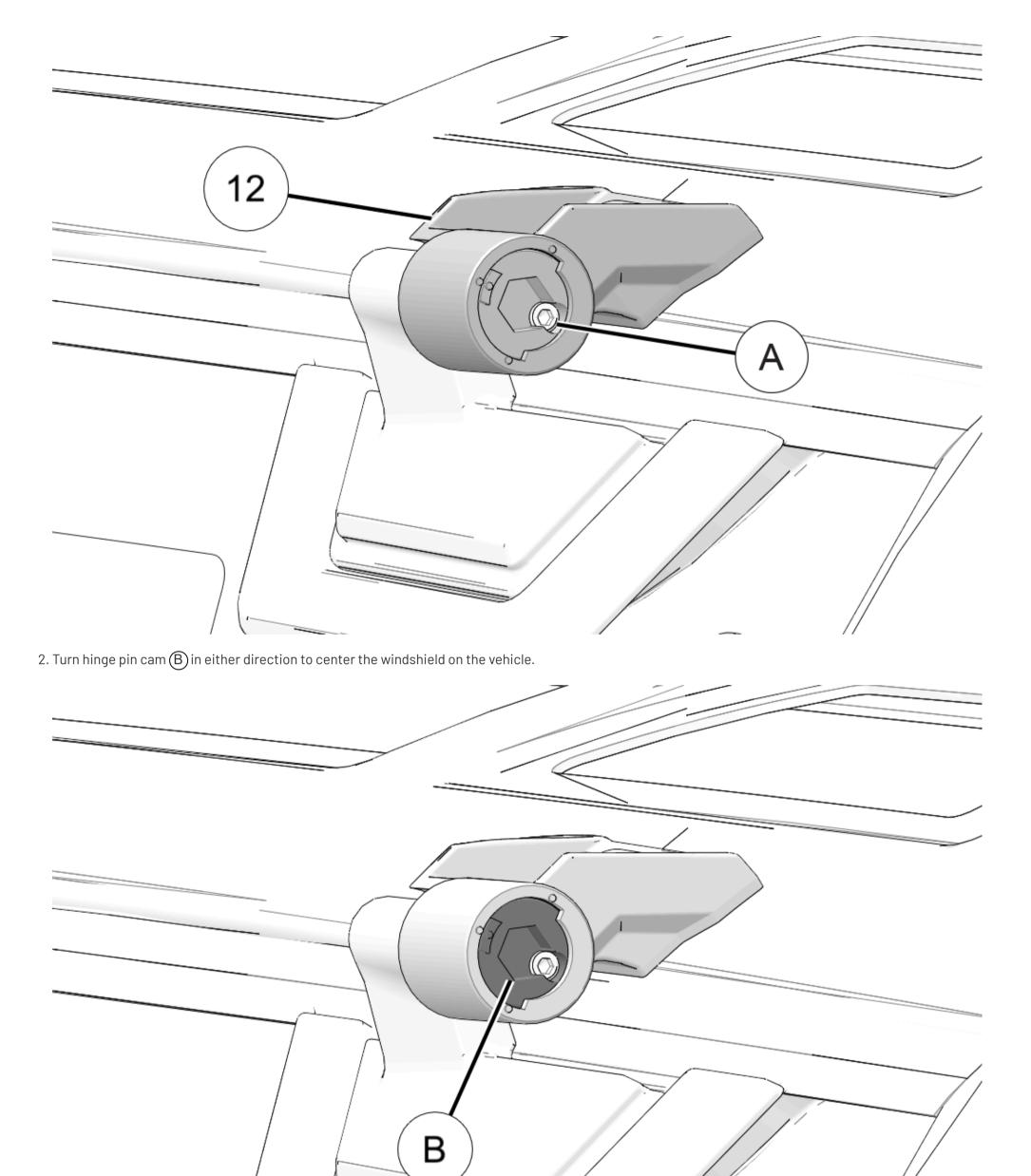
3. Tighten set screw (A) on left side windshield mount (12).
