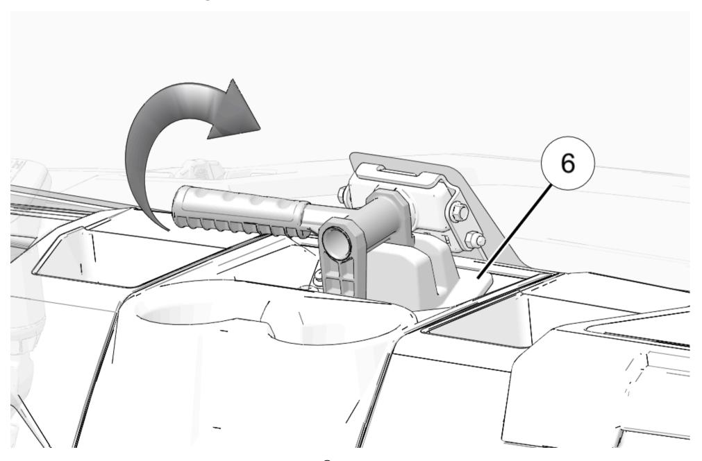
2. Move windshield handle forward and align handle legs over handle base 6 in the vented position, as shown.
