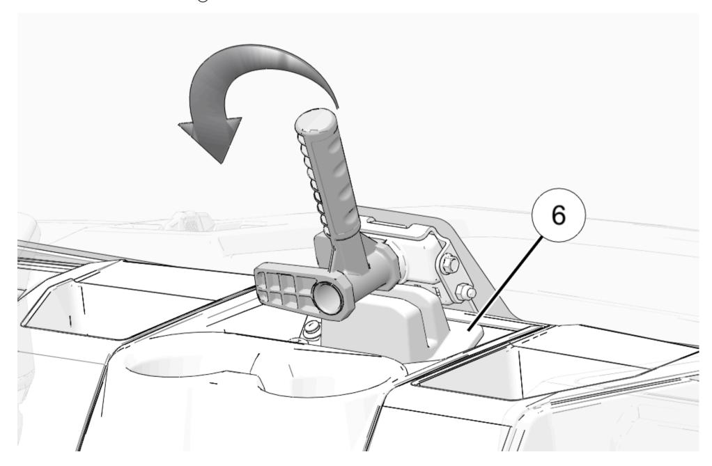
3. Make sure windshield seals are compressed and that the windshield opens and closes correctly. See Windshield Alignment section if adjustments are needed.
