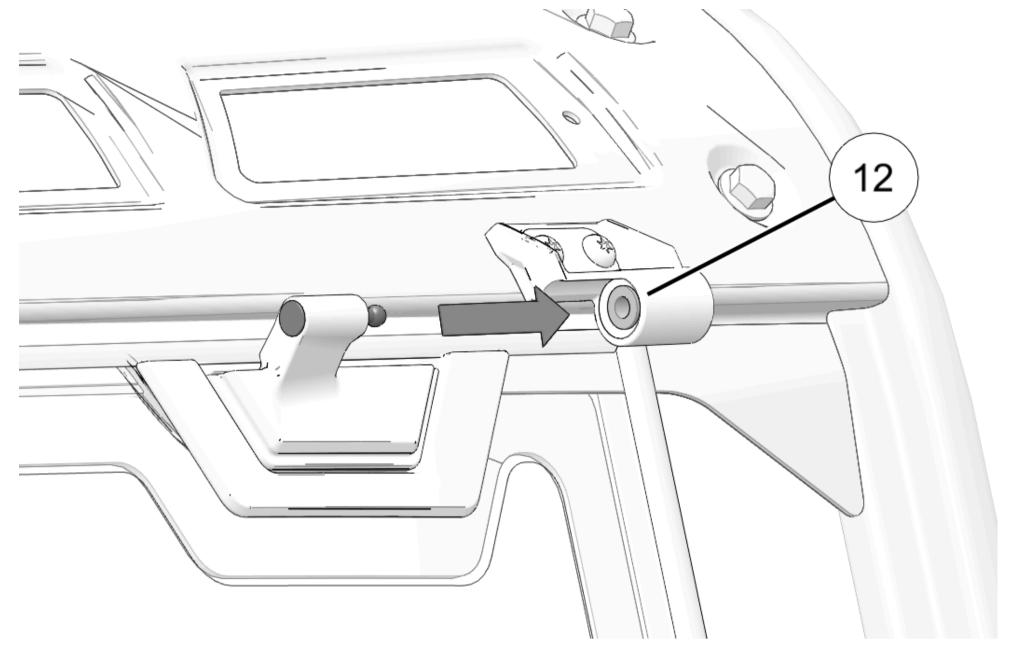
4. Install right side windshield mount bushing 11 onto right side windshield hinge pin.
