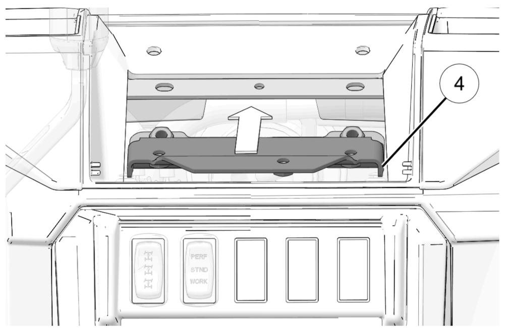
2. Install backer bracket 4 to upper chassis bar with two screws 5.
