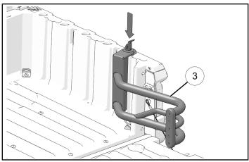
4. Align Lock & Ride® anchor of the left-hand extender ② with the rearmost hole in the cargo box.
