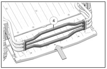
7. Loosely install each side of the center assembly with two bolts ③ and two nuts ⑦.
