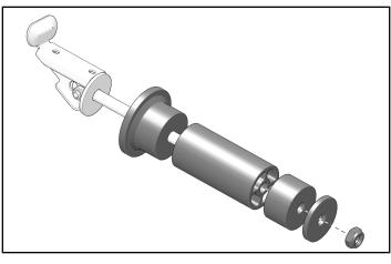
2. Assemble Lock & Ride® anchors ① onto the lefthand extender ② and the right-hand extender ③. Make sure the washer is on top of the extender, as shown.
