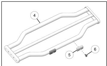
6. Put the center assembly 4 on the tailgate between the right and left extenders.
