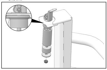
3. Align Lock & Ride® anchor of the right-hand extender ③ with the rearmost hole in the cargo box.
