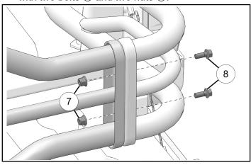
8. Counter-hold the nut ① and torque each bolt ⑧ to specification.
