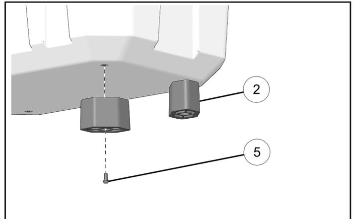
5. Lock & Ride® assemblies may require adjustment. Adjust fitment by tightening or loosening bottom nut.
