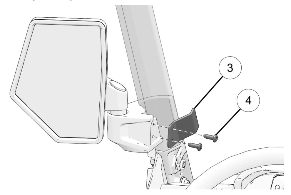
3. Tighten screws until fully seated.
