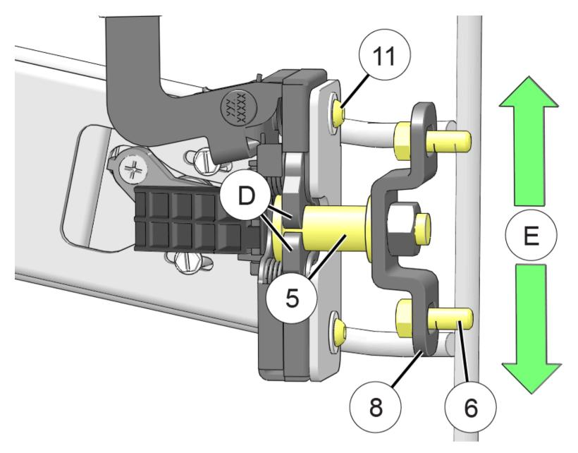
3. **DEPTH** (F): As required to achieve desired fairing between door frame (1) and ROPS/chassis door structure. To adjust, loosen two screws (6), slide striker bracket (8) inboard or outboard as required, then retighten screws.
