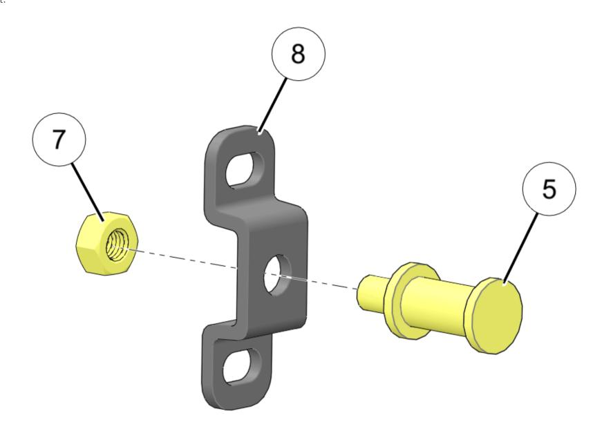
16. Install striker bracket (8) to chassis structure using two screws (8). Center striker over screw holes in chassis, then partially tighten screws.
