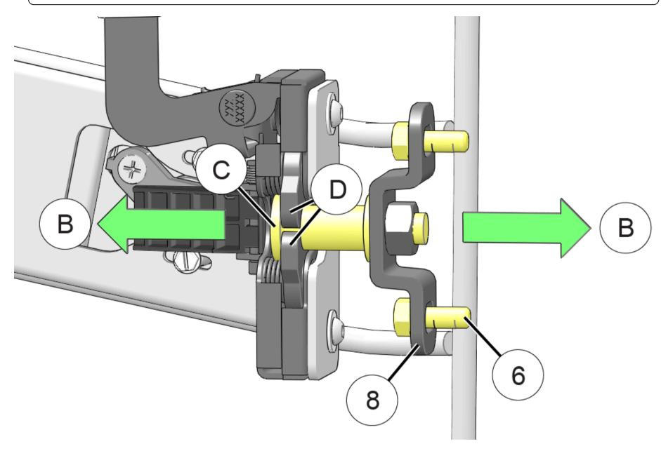
2. **HEIGHT** (E): Pin (5) should be centered vertically in opening of latch pawls (D). To adjust, loosen two screws (6), slide striker bracket (8) up or down as required, then retighten screws.
