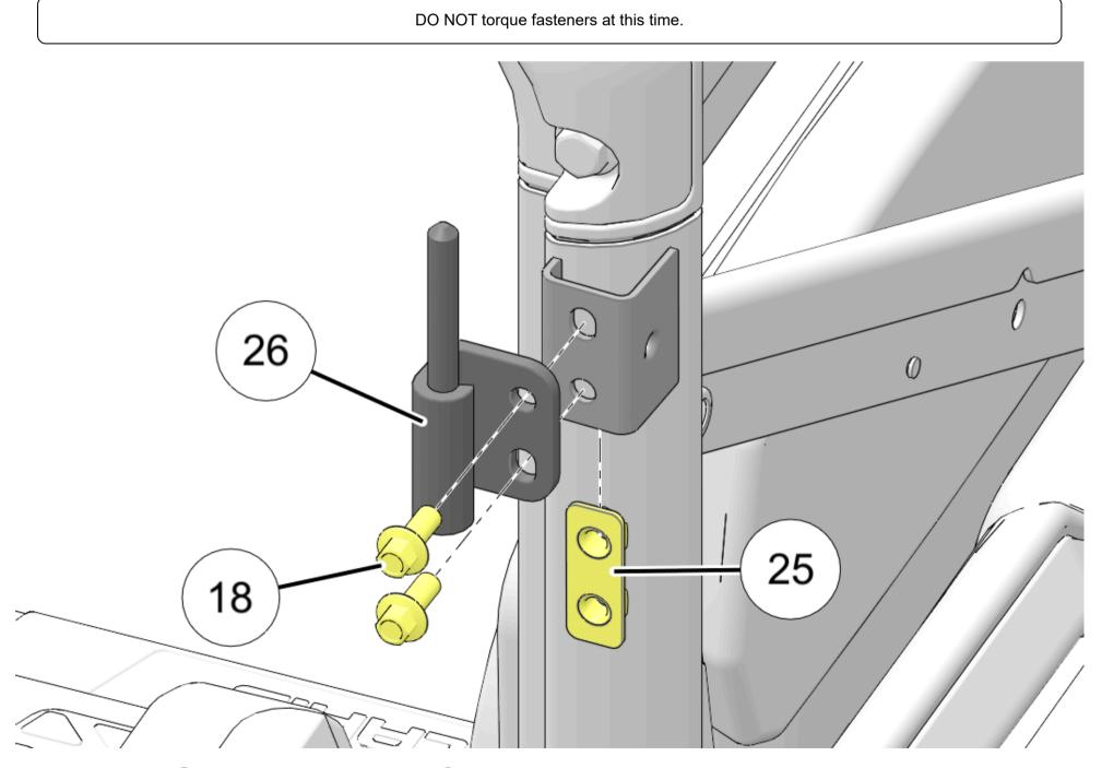
6. Install lower left hinge 19 to chassis using two each screws 18. Center hinge over screw holes in vehicle, then partially tighten screws.
