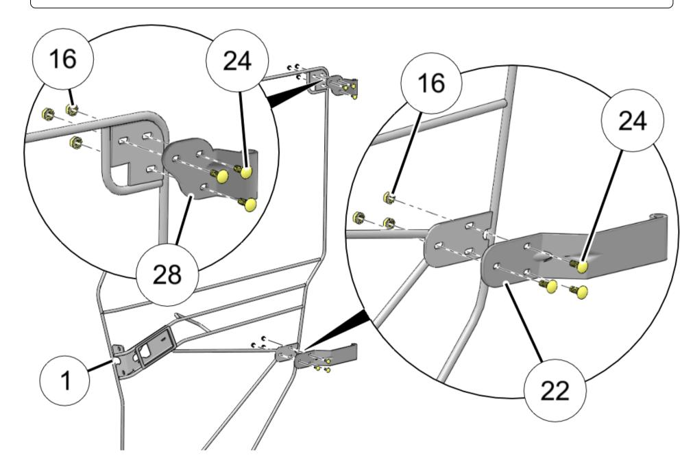
4. Loosely install lower left door side hinge (22) to left door frame (1) using three each carriage bolts (24) and nuts (16).
