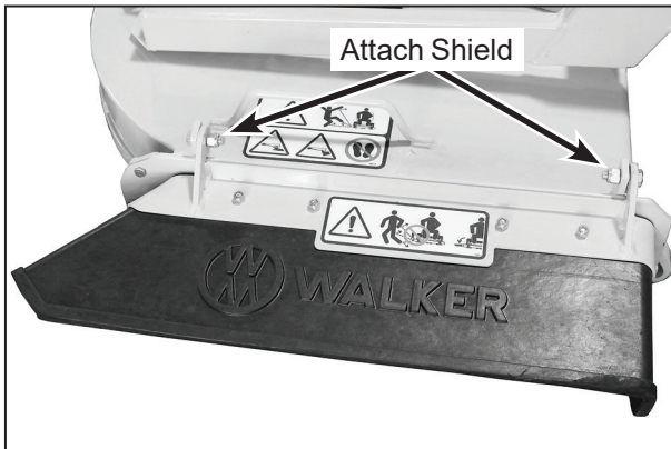
Deck Discharge Shield Installation
