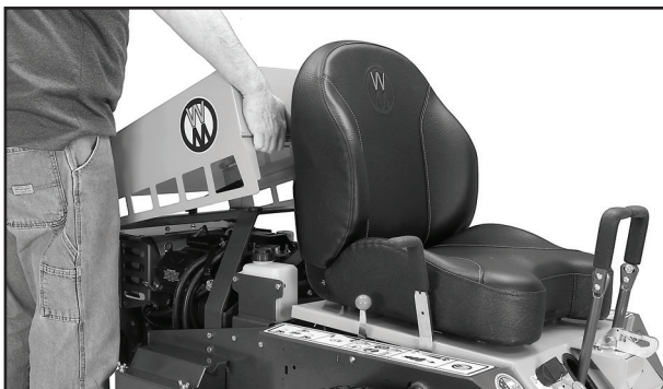
Lifting Rear Body (Optional Dump Bed Shown)
