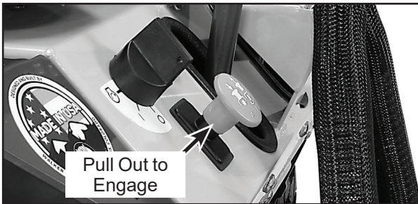
Blade Clutch Engaged
