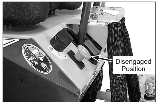
Blade Clutch Disengaged
